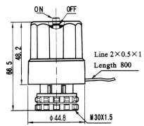
The product shown is normally close. When power are given, the position will be ON, if cut the power the Position will be OFF.
